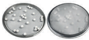
Elastomeric balls anti-blinding device
